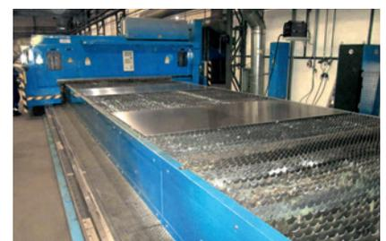
Laser cutting plant for the extraction of steel and aluminum dust, which need to be removed during the cutting of ship components.
