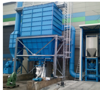
Bag filter system from Entstaubungstechnik Schwarzenberg for arresting foundry dusts
